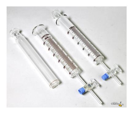
The tip of the syringe is connected to the apparatus via gas tubing or pierced stoppers.
