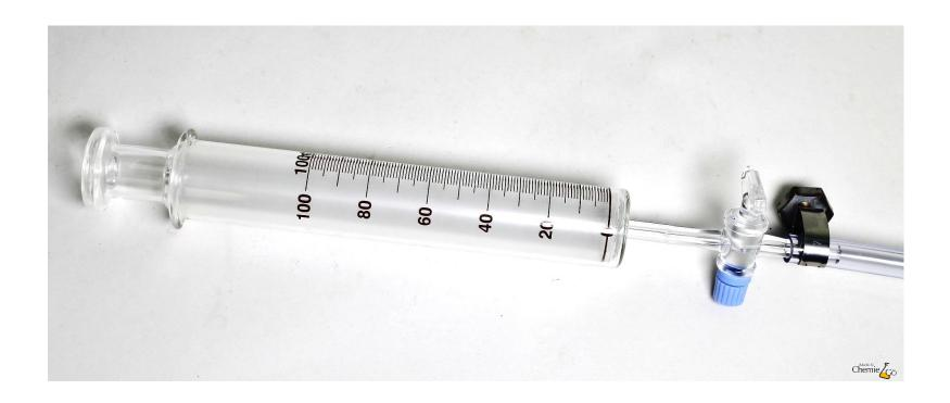
The volume of gas in the syringe can be determined via the mark on the plunger.
